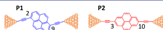
Figure 1. Two molecules P1 and P2 with common pyrene hearts but different connectivities to gold electrodes. (See Figure 2 for more details of the numbering convention used in this study. This does not correspond to the usual chemical numbering convention, but it is convenient analytically and allows us to assign labels to all atoms.)
